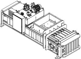
Installation would include the hiring of a construction firm to lift the baler off the shipping flat, move it to its designated place of operation, anchoring it into the concrete, installing any attachments that were removed for shipping, connecting all electrical equipment (disconnect and conduit), and installing hydraulic oil if it was removed for shipping. If a new unit is purchased, final electrical connections and training from the sales staff comes with the purchase.
