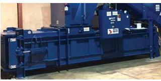
Installation would include the hiring of a construction firm to lift the baler off the shipping flat, move it to its designated place of operation, anchoring it into the concrete, installing any attachments that were removed for shipping, connecting all electrical equipment (disconnect and conduit), and installing hydraulic oil if it was removed for shipping. If a new unit is purchased, final electrical connections and training from the sales staff comes with the purchase.
