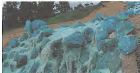
Cullet from the Pittsburgh Plate Glass plant
