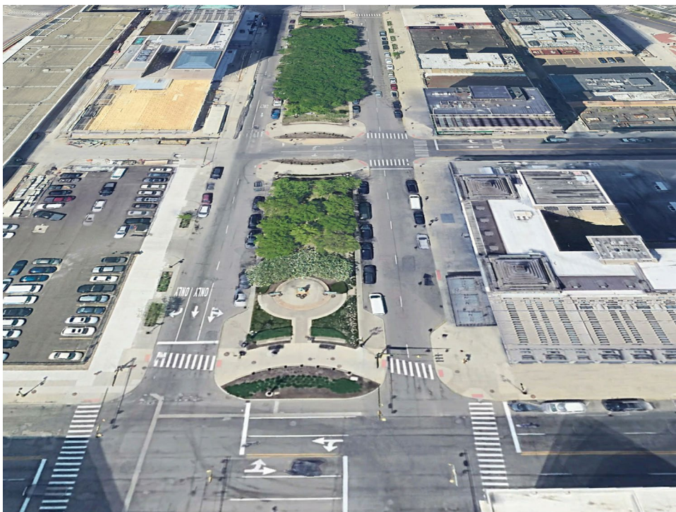
Examples of on-street parking lanes adjacent to medians in Detroit, MI (top: Anthony Wayne Drive, bottom: Washington Boulevard).
