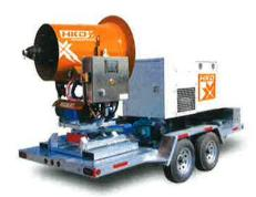
The Super Blizzard includes a pump, HKD Turbo fan, and 65 KVA generator - all mounted on a 16' trailer. This machine is ready to tackle bury your toughest snowmaking project.
