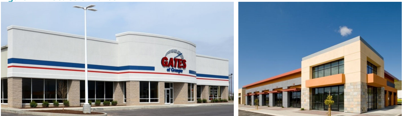
Left: Color bands without change in plane or materials. Right: Color bands using different planes.
