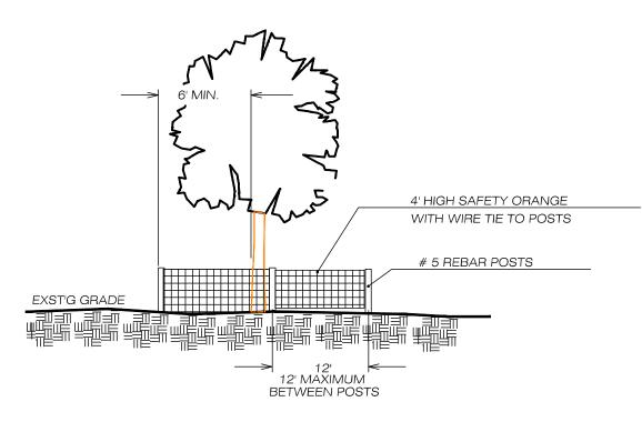
TREE PROTECTION DETAIL PLACE TREE PROTECTION BARRIER AROUND ALL TREES SHOWN TO REMAIN WITHIN CONSTRUCTION AREAS
