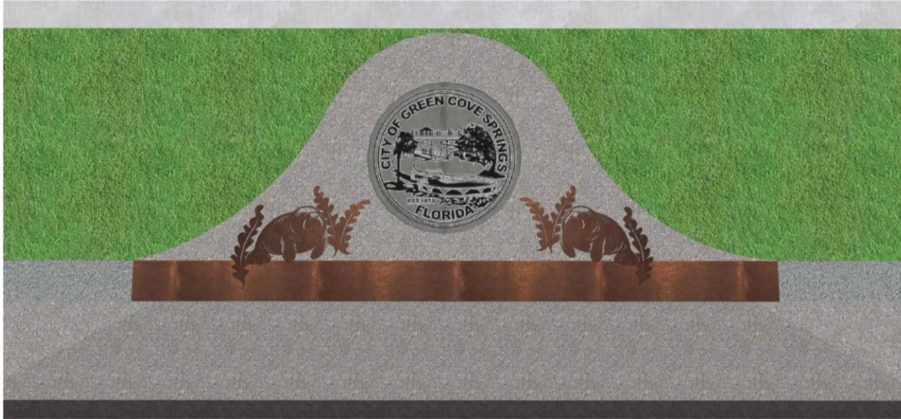
**Copper manatees are inlaid on top of storm drain with copper edge at the curb opening.**
