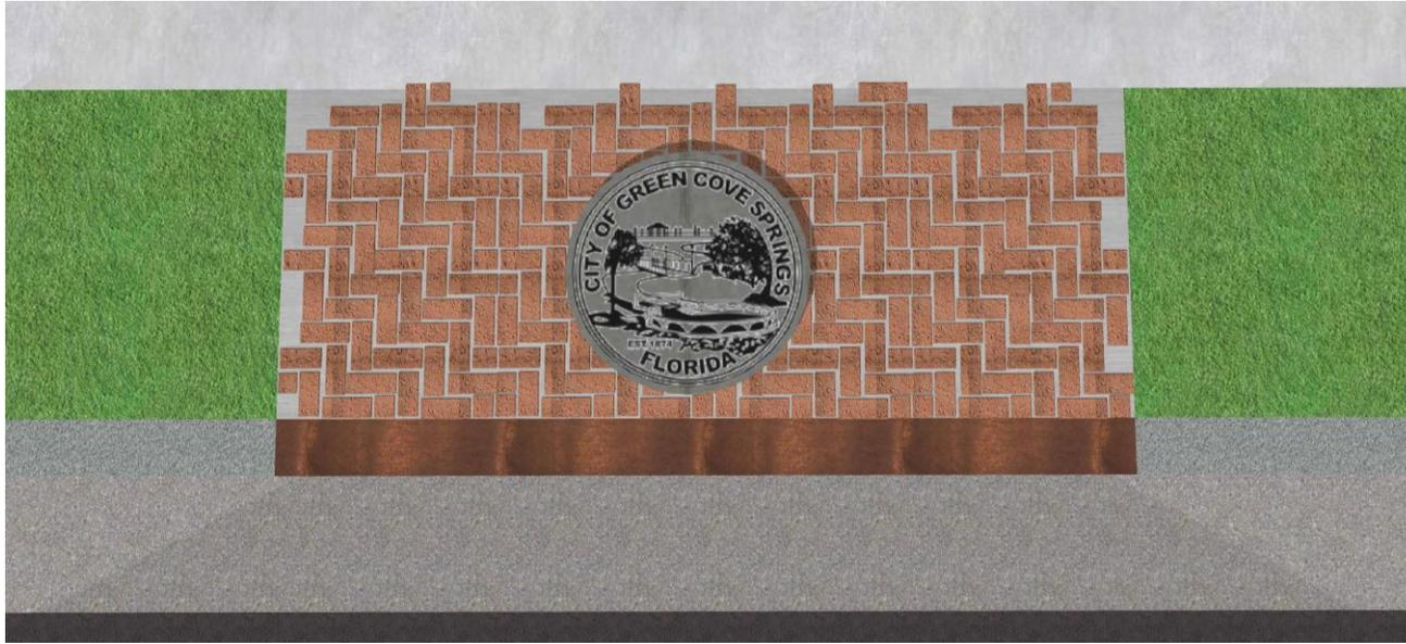
Old brick pattern is stamped on concrete with a copper edge at the opening of the drain.
