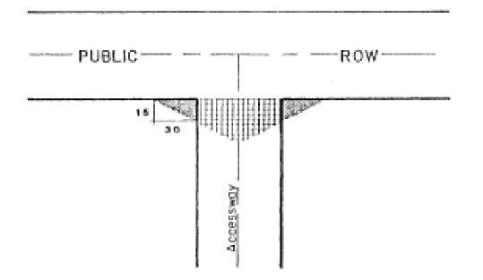
(b) The area of property formed by the intersection of an accessway and a public right-of-way with one (1) side of the triangular area being thirty (30) feet in length along the public road right-of-way line measured from the edge of the accessway pavement and one (1) side of the triangle being fifteen (15) feet in length along the accessway pavement measured from the public road right-of-way line, and the third side being a line connecting the ends of the other two (2) sides.
