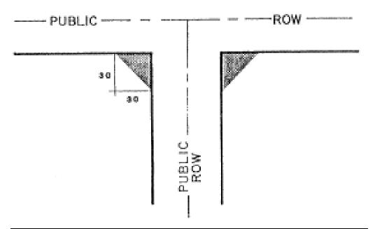
(c) The area of property formed by the intersection of two (2) accessways with two (2) sides of the triangular area being a minimum of fifteen (15) feet in length along the accessway pavement, measured from their point of intersection, and the third side being line connecting the ends of the other two (2) sides.
