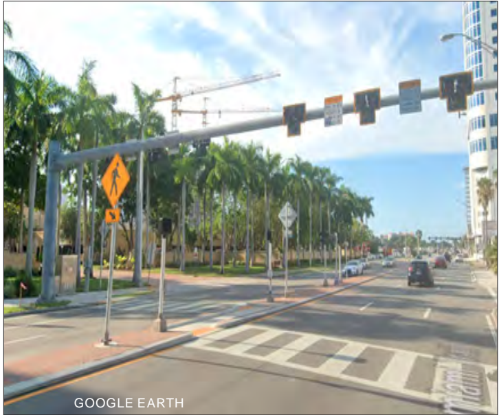
HAWK SIGNAL MID-BLOCK PROVIDING PEDESTRIAN REFUGE & ACCESS
