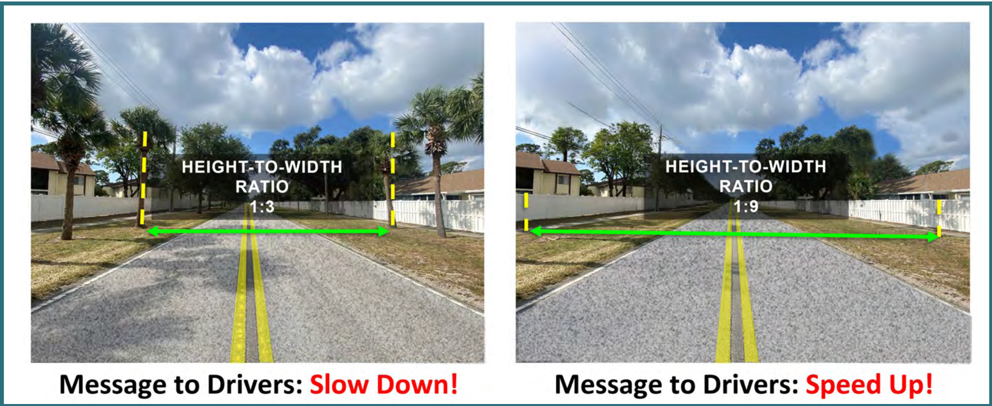
Figure 45 Height-to-width comparison of the relationship between street trees and a sense of enclosure; Sherwood Forest Boulevard modeled as typical Greenacres condition
