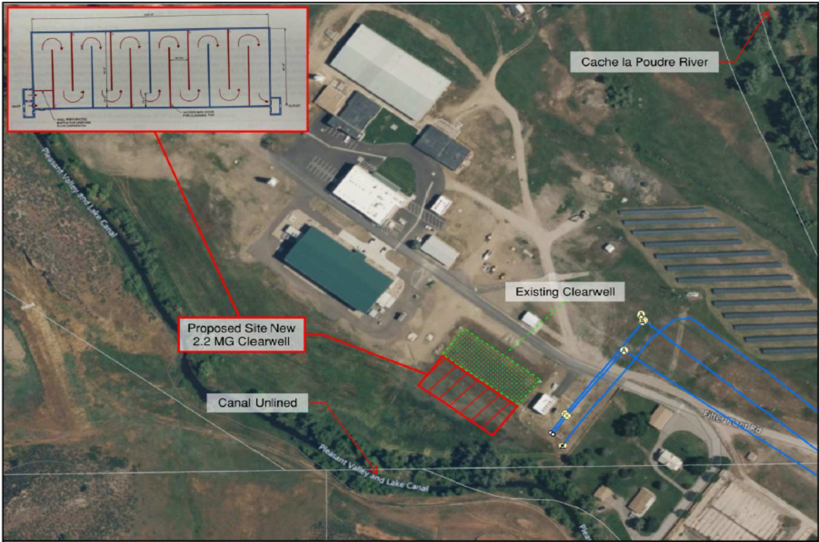
Bellvue Water Treatment Plant - 2.2 MG Clearwell
