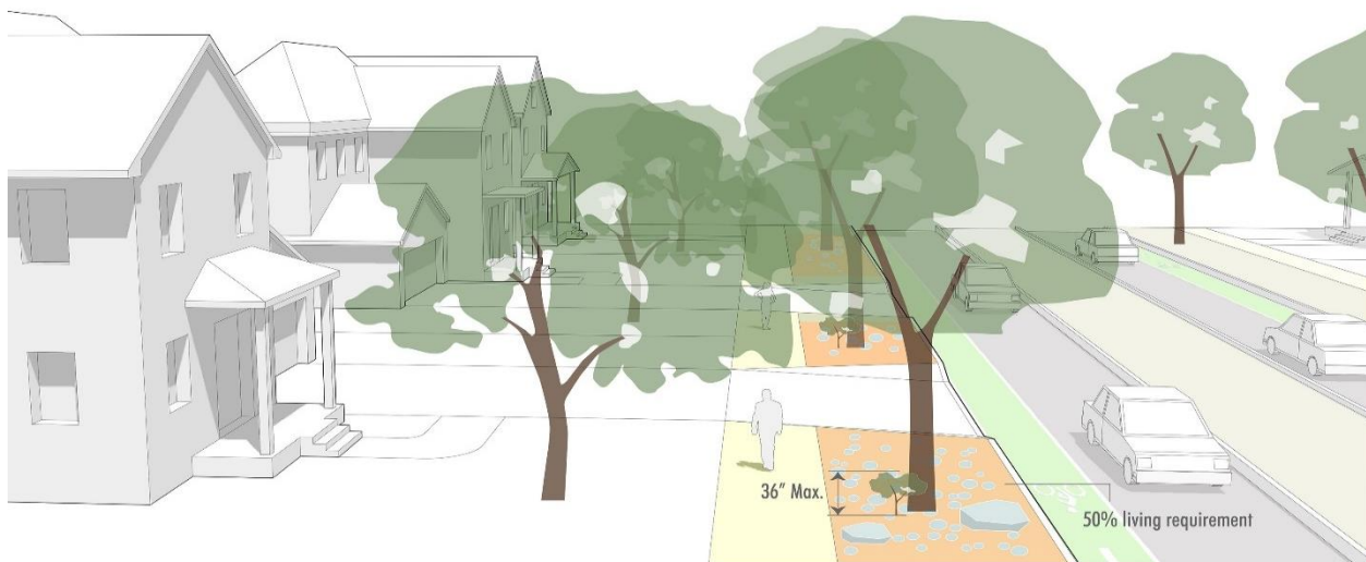
Figure 18.44-5b: Tree sidewalk clearance - residential
