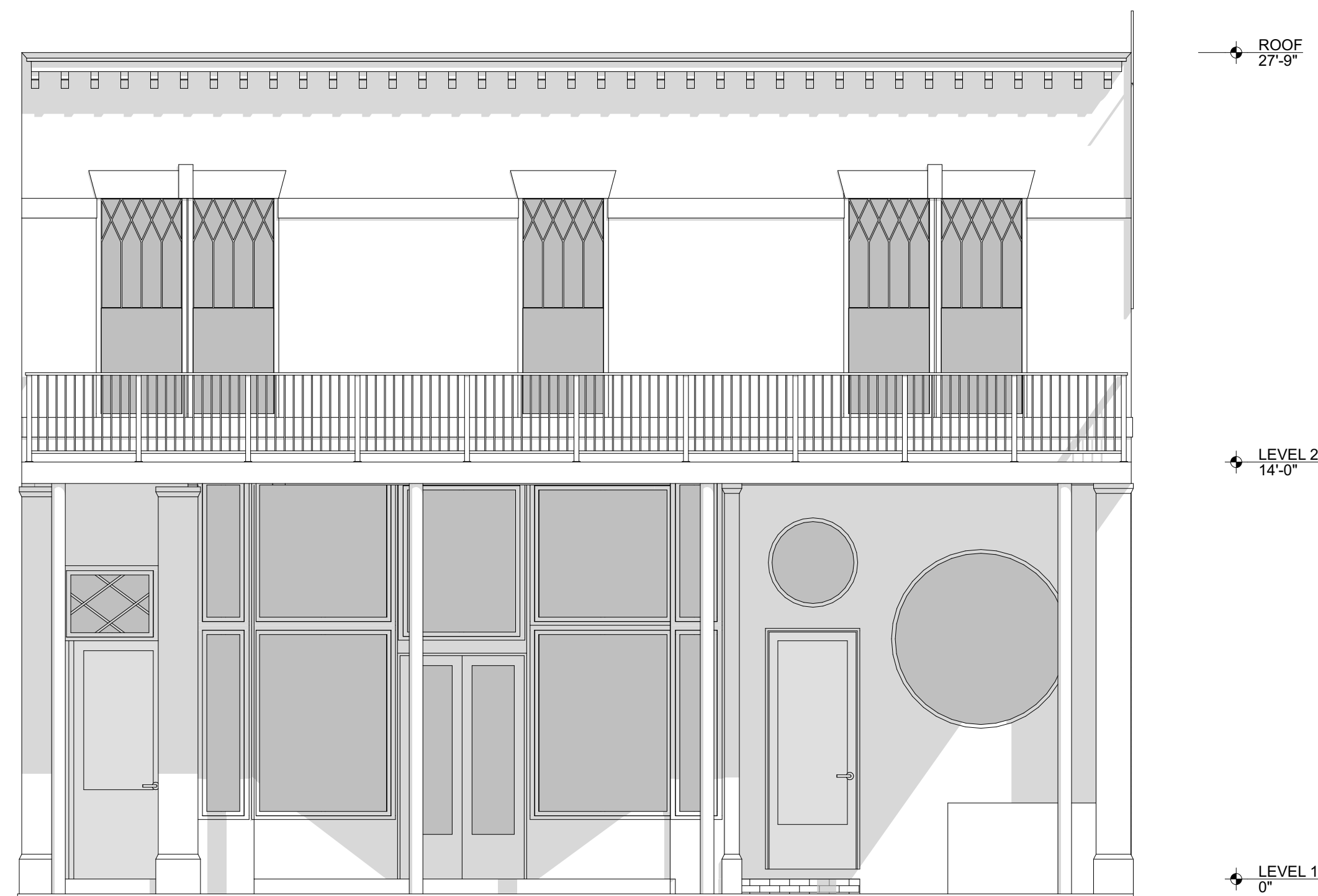
4 WEST ELEVATION (MILL ST.) - EXISTING SCALE: 1/4" = 1'-0"
