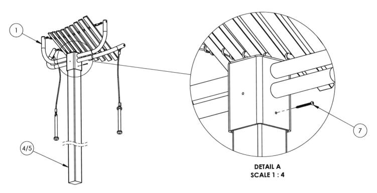
**Step 1:** Excavate one 10" diameter hole, 36" deep, at the installation location. Contractor can modify Post to desired height.
