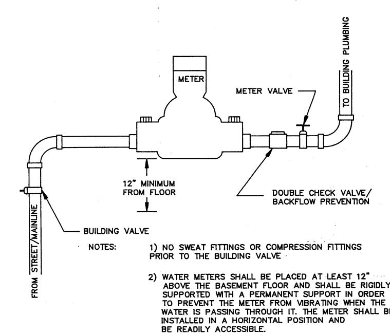
TYPICAL WATER METER INSTALLATION
