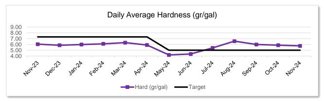
Due to the disinfection, water softening was increased to enhance corrosion protection measures.
