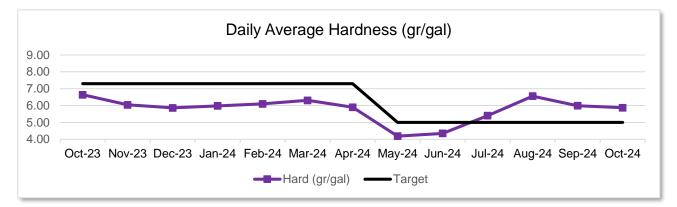
Due to the disinfection, water softening was increased to enhance corrosion protection measures.
