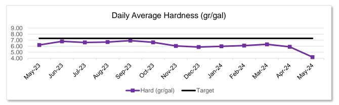
Due to the upcoming disinfection, water softening was increased to enhance corrosion protection measures.
