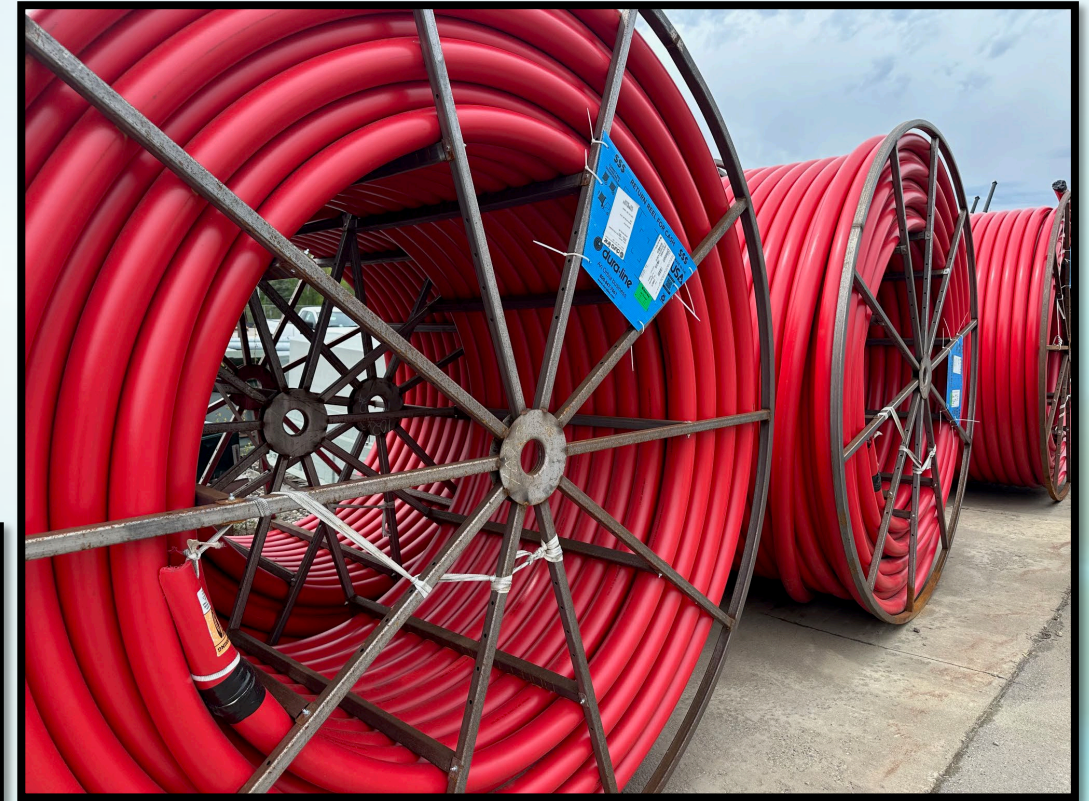
Innerduct – Bored in then cable is pulled inside
