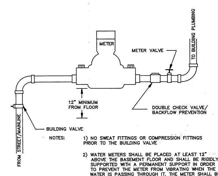
TYPICAL WATER METER INSTALLATION
