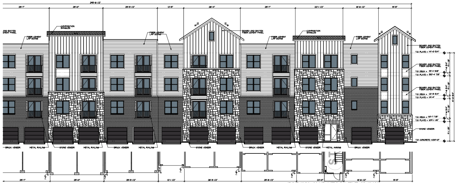
01 PARTIAL NORTHEAST ELEVATION BUILDING 300 SCALE: 1/8"=1'-0"
