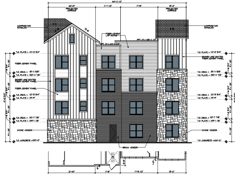
02 SOUTH ELEVATION BUILDING 100 SCALE: 1/8"=1'-0"
