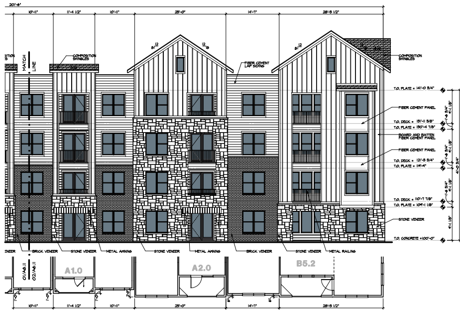
02 PARTIAL SOUTH ELEVATION BUILDING 300
