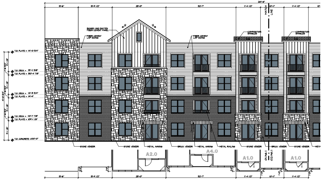
01 PARTIAL SOUTH ELEVATION BUILDING 300
