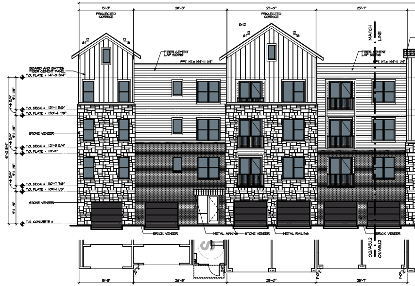
02 PARTIAL SOUTH COURT ELEVATION BUILDING 200 SCALE: 1/8"=1'-0"
