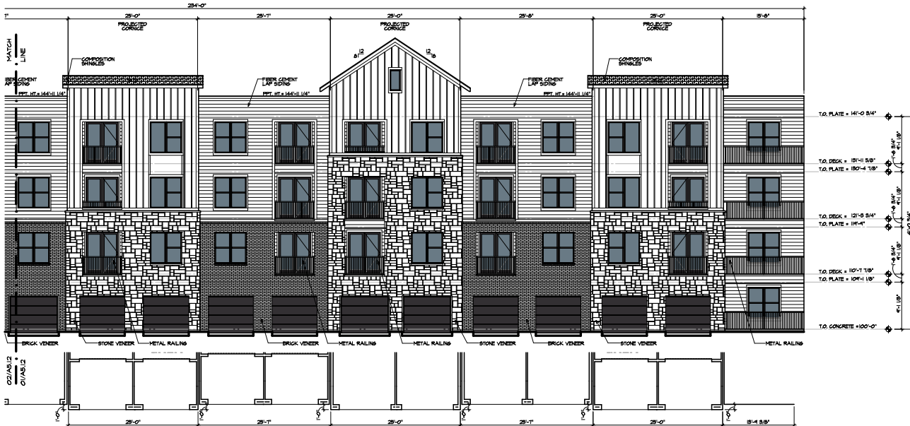
01 PARTIAL SOUTH COURT ELEVATION BUILDING 200 SCALE: 1/8"=1'-0"
