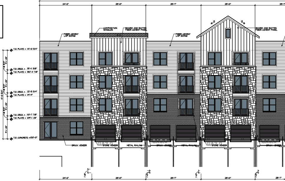
02 PARTIAL NORTHEAST ELEVATION BUILDING 300 SCALE: 1/8"=1'-0"
