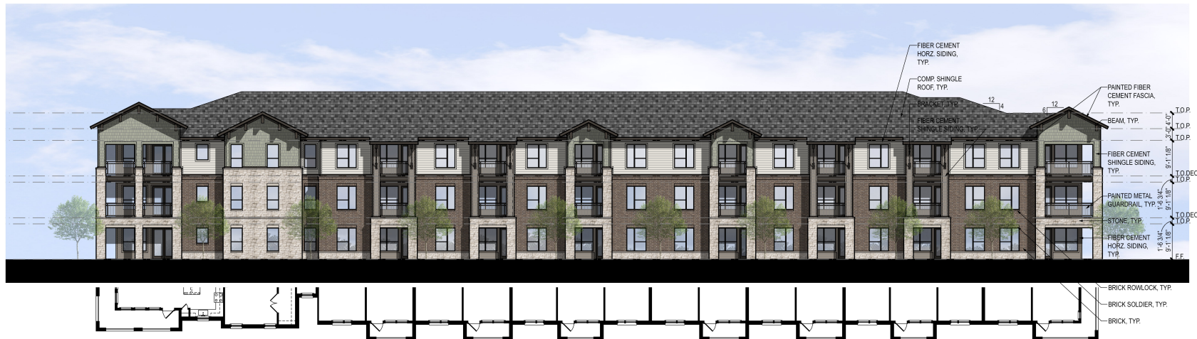
CONCEPT BUILDING ELEVATION ALONG STATE HIGHWAY 360 1 SC: 3/32" = 1'-0"
