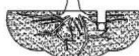
OPEN TRENCHING MAY BE USED IF EXPOSED TREE ROOTS DO NOT EXCEED 3" OR ROOTS CAN BE BENT BACK.
