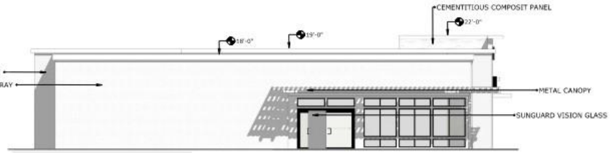
02 BUILDING A- SOUTH ELEVATION (LEFT) SCALE 1/8"=1'-0"
