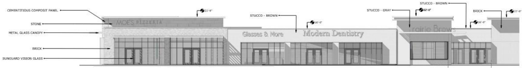
01 BUILDING B- EAST ELEVATION (FRONT) 1-2 SCALE 1/8"=1'-0"
