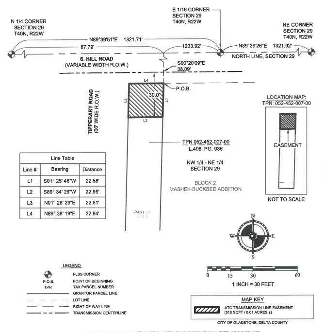
NOTE - BEARINGS ARE BASED ON THE MICHIGAN STATE PLANE COORDINATE SYSTEM, NORTH ZONE, INTERNATIONAL FEET, GRID DISTANCE.
