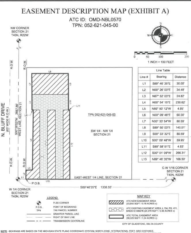
NOTE - BEARINGS ARE BASED ON THE MICHIGAN STATE PLANE COORDINATE SYSTEM, NORTH ZONE, INTERNATIONAL FEET, GRID DISTANCE.
