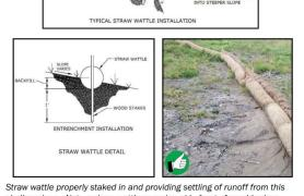
shallow slope. Note a clean wattle was placed in front of an older less effective wattle. Install Perimeter Controls
