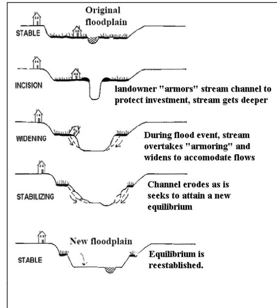
**Figure 3.27: Fluvial Erosion**
