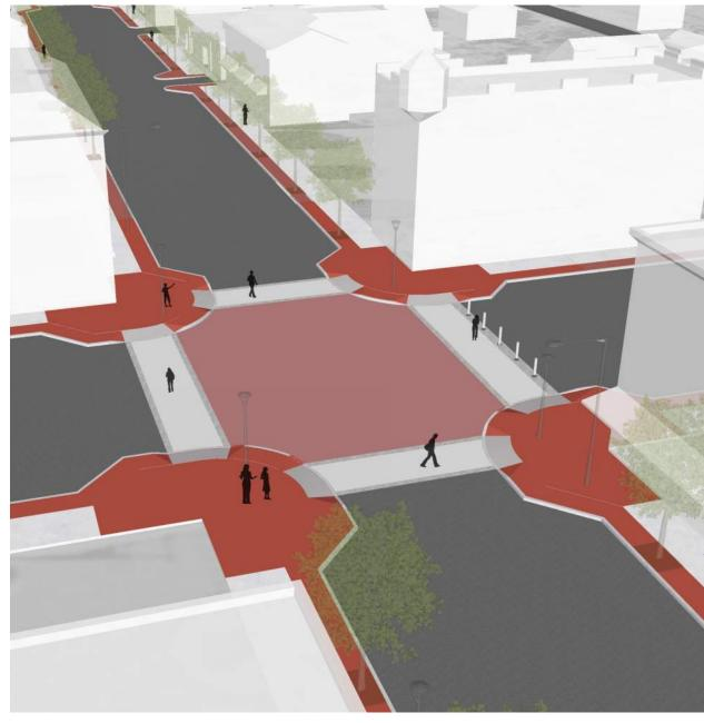
4' BRICK UTILITY STRIP | BRICK AT INTERSECTION BUMP OUT | CONCRETE SIDEWALK
