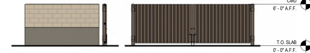
5 TRASH ENCLOSURE ELEVATIONS Scale: 1/8" = 1'-0"
