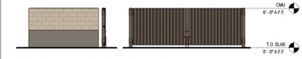
5 TRASH ENCLOSURE ELEVATIONS Scale: 1/8" = 1'-0"
