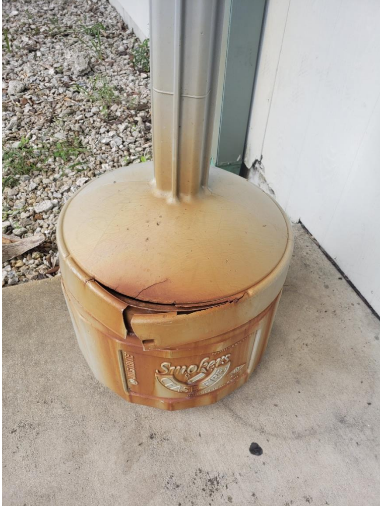
Cigarette receptacle fire damage
