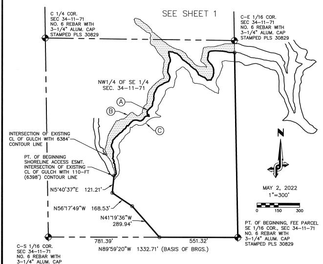
NOTE: 110-FOOT CONTOUR HAS BEEN DETERMINED TO BE AT NAVD 88 ELEVATION 6398' THROUGH 1) THE RECOVERY AND GPS SURVEY OF THE BENCHMARK MARKED "ELEVATION 76.47" ESTABLISHED IN 1910 AND SHOWN ON THE 'MAP OF RESURVEY OF THE HALLIGAN RESERVOIR', AND 2) THE SURVEY OF THE SPILLWAY WHOSE ELEVATION IS 70' AS INDICATED ON SAID MAP.
