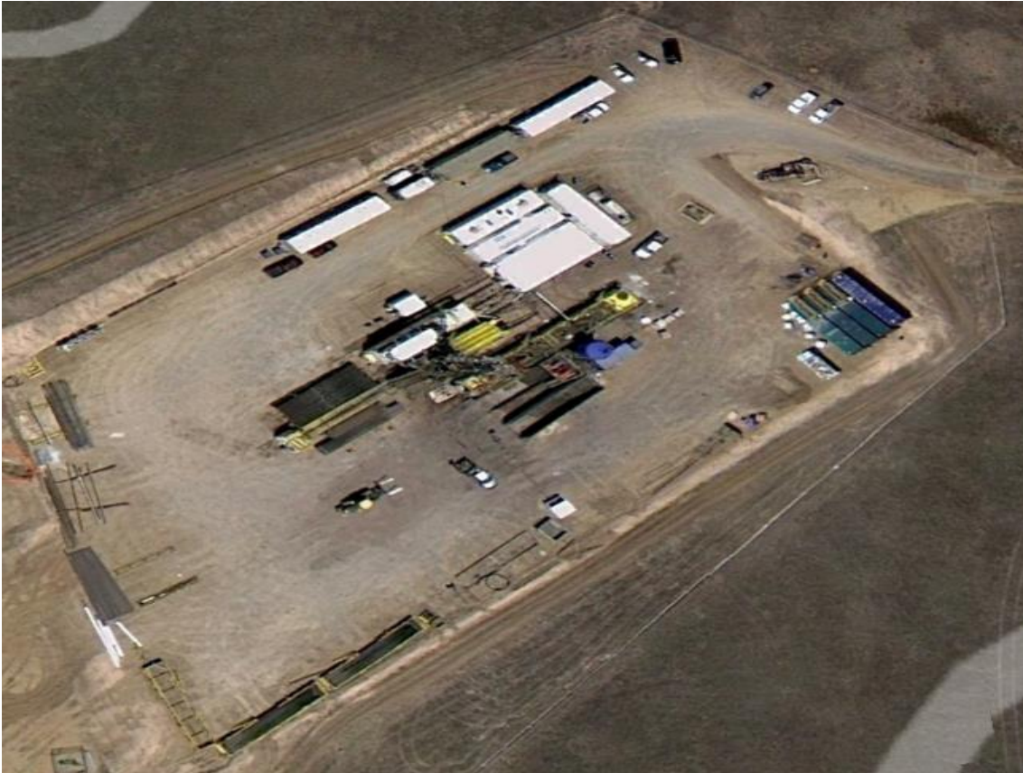
Figure 3: Google Earth image of a vertical well drilling in 2011 on 2-acres in Weld County.
