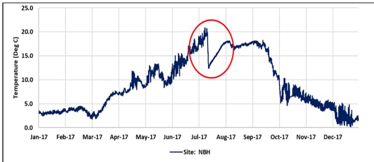
Figure C-8. Example of Thermal Shock below Halligan Dam (NBH), 2017
