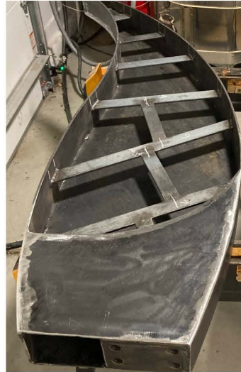
Steel support bars welded to sculpture.
