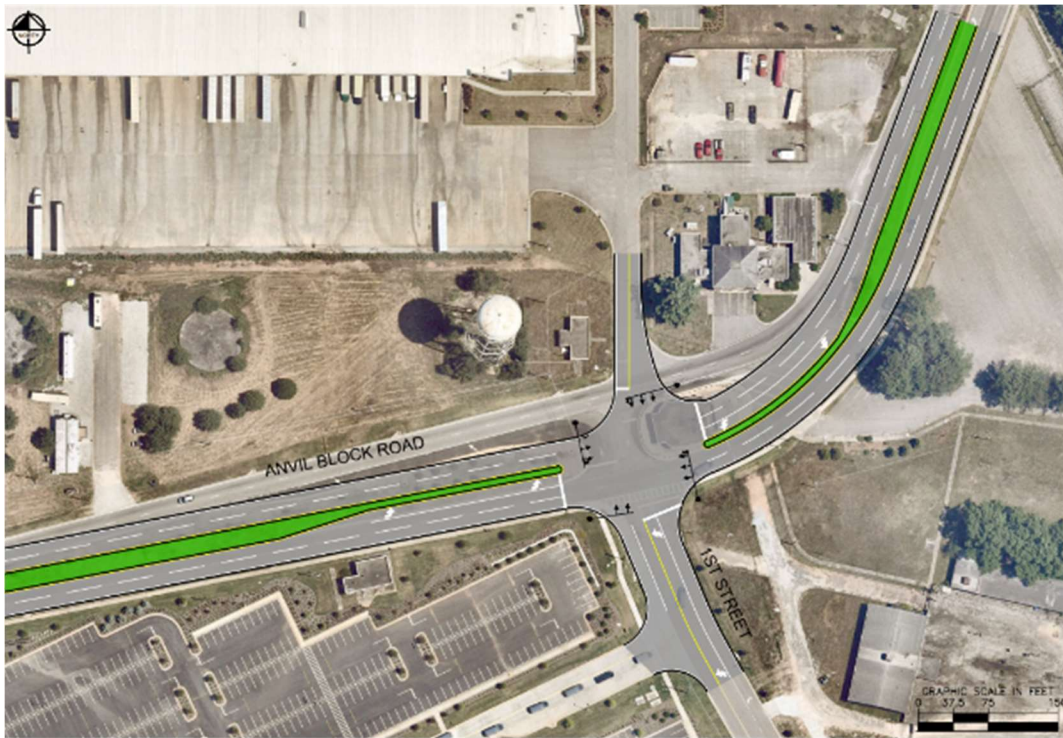
Figure 2: Alternative 2 - Traffic Signal with Realignment
