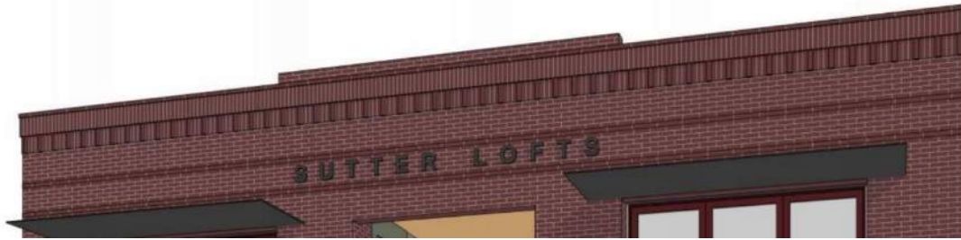
Figure 4 – Proposed Cornice on Parapet
