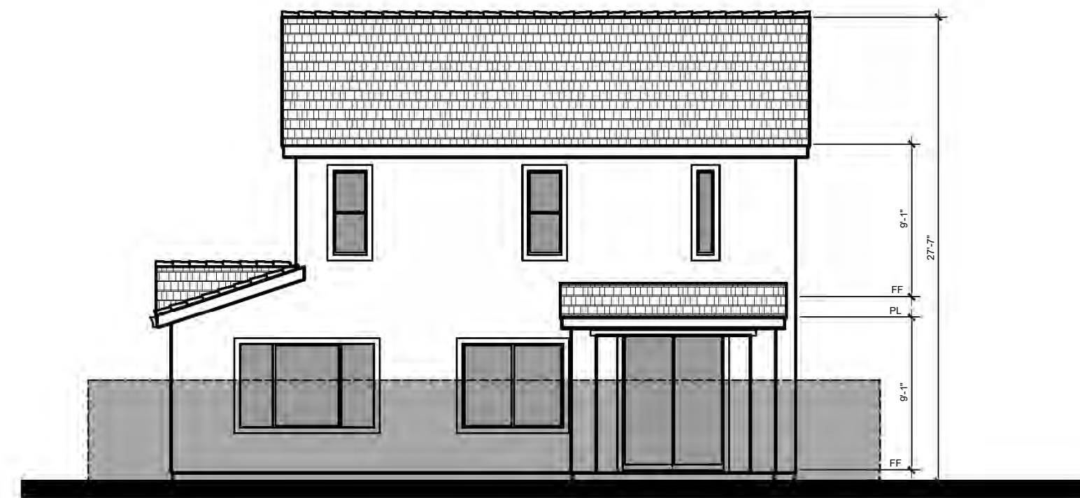
Rear Elevation - 2B Opt. Covered Outdoor Room
