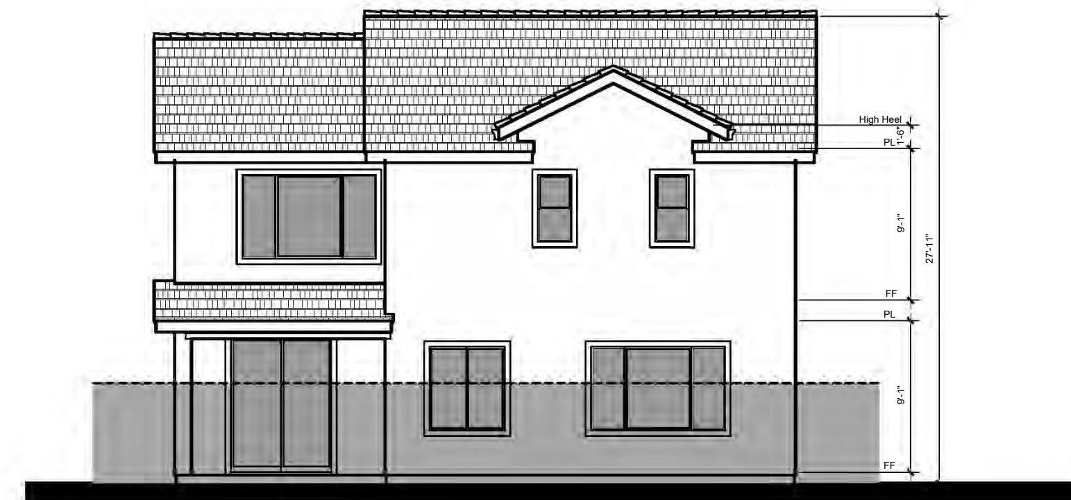
Rear Elevation - 1B Opt. Covered Outdoor Room
