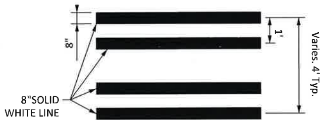
ENTRY BUFFER STRIPING DETAIL N.T.S.
