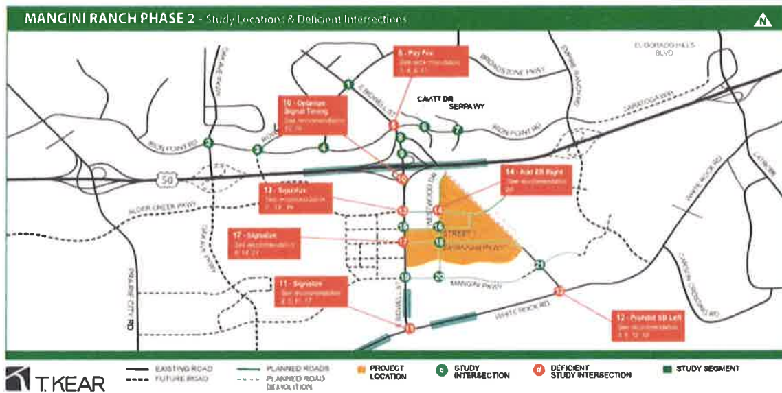
Figure ES-2. Study Locations, Deficiencies, And Recommendations
