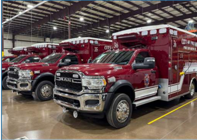
Photo of Type 1 ambulances lined up side by side inside the Fire Station
