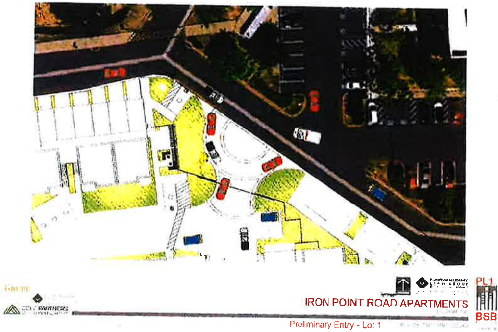
Figure ES-3. Entry Gate Detail At For "Lot 1" (Western Portion Of Project) Showing Queue Storage At Entry Gate
