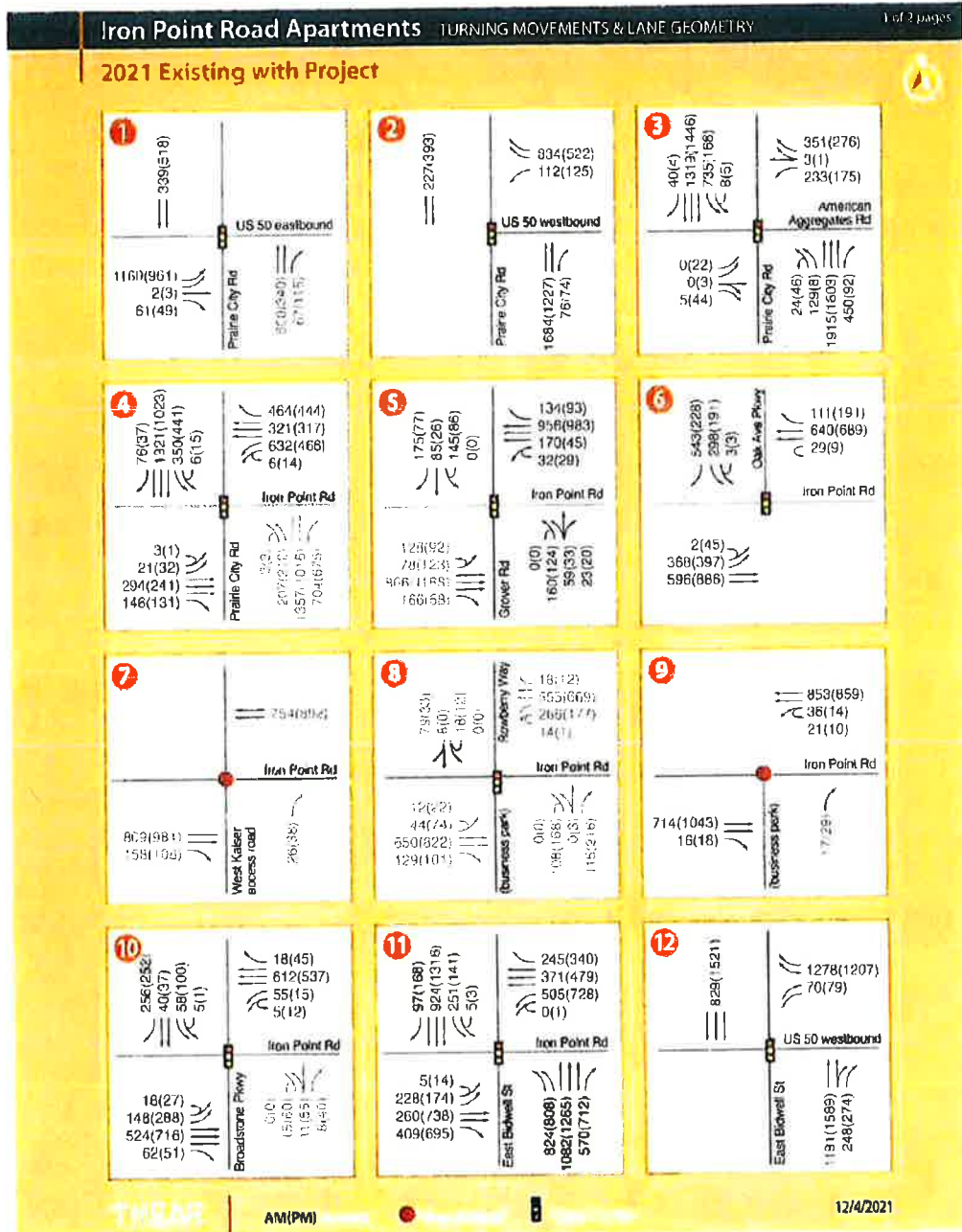
Figure 16. Existing 2021 with Project Condition Turning Movements and Lane Geometry
