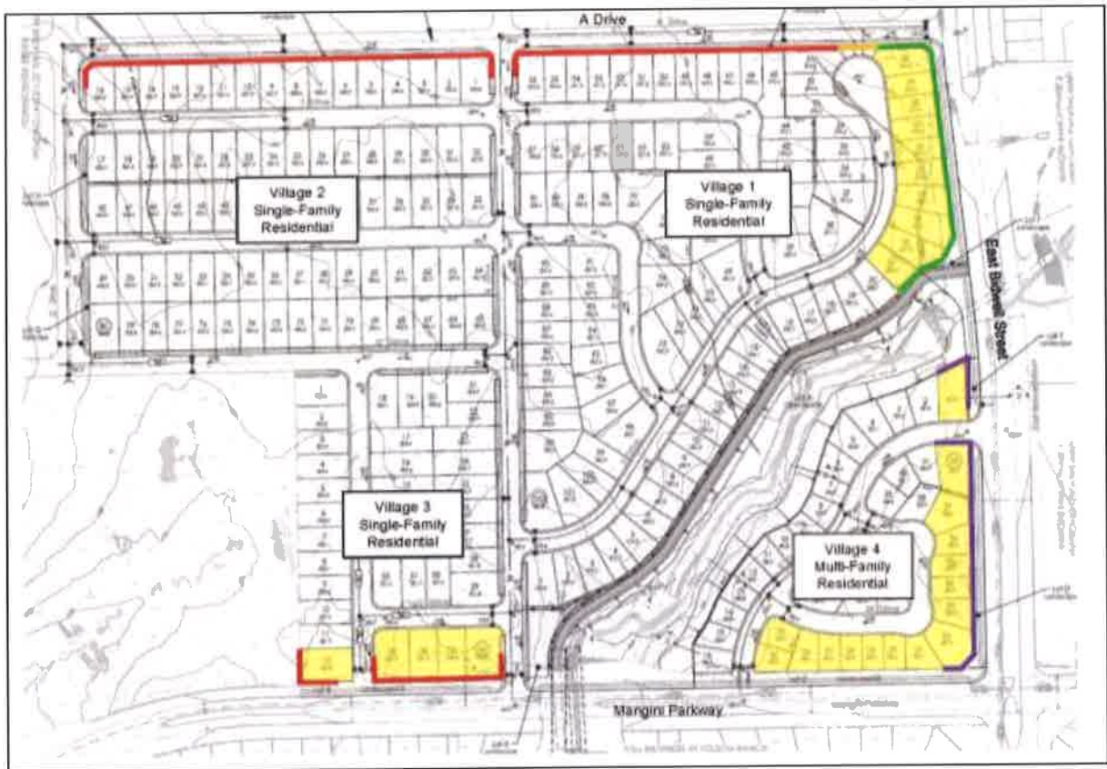
FIGURE 12: RECOMMENDED SOUNDWALL LOCATIONS
