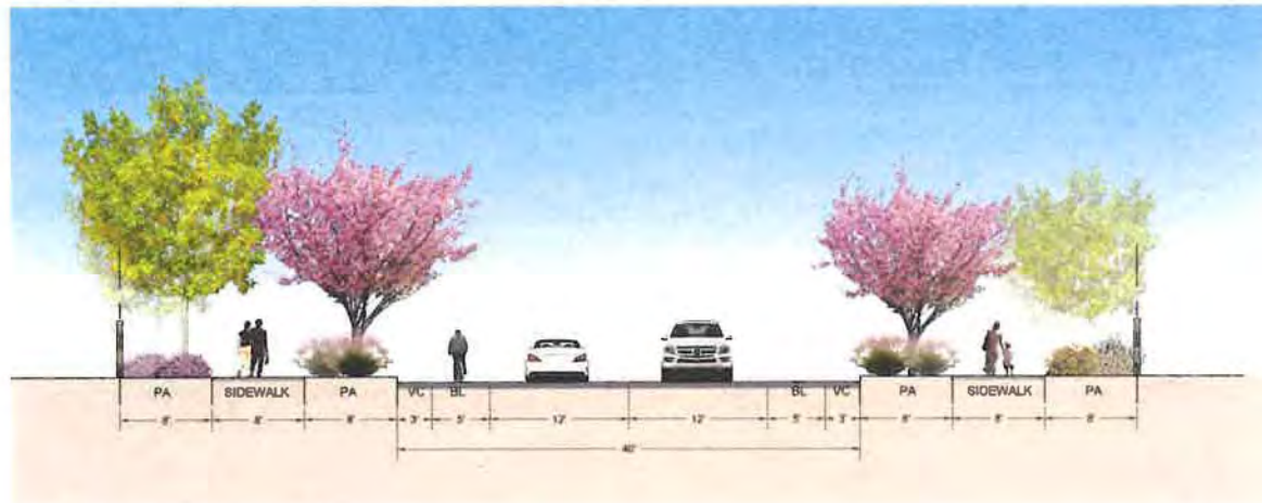
REGENCY PARKWAY CROSS SECTION SCALE: 3/16"=1'-0"
