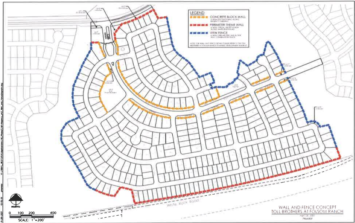
FIGURE 8: WALL AND FENCE EXHIBIT
