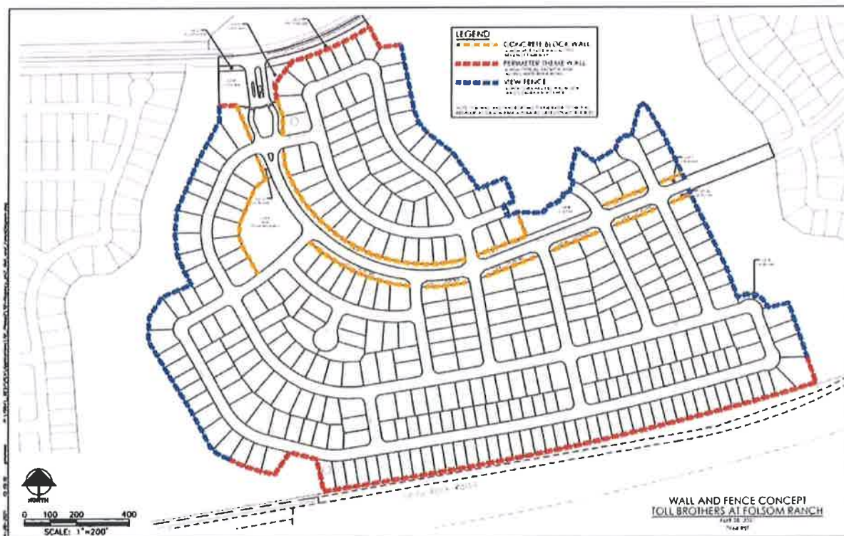
Figure 9: WALL AND FENCE EXHIBIT
