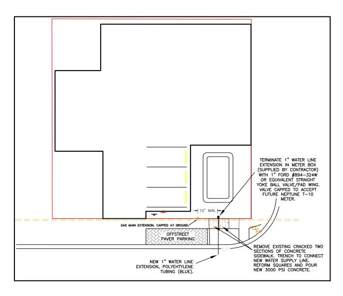
WATER & SEWER CONNECTION DETAIL
