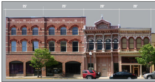
Figure 7-3 Illustration showing building articulation requirement
