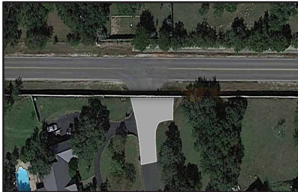
Figure 22 – Partial Hammerhead Turnaround
