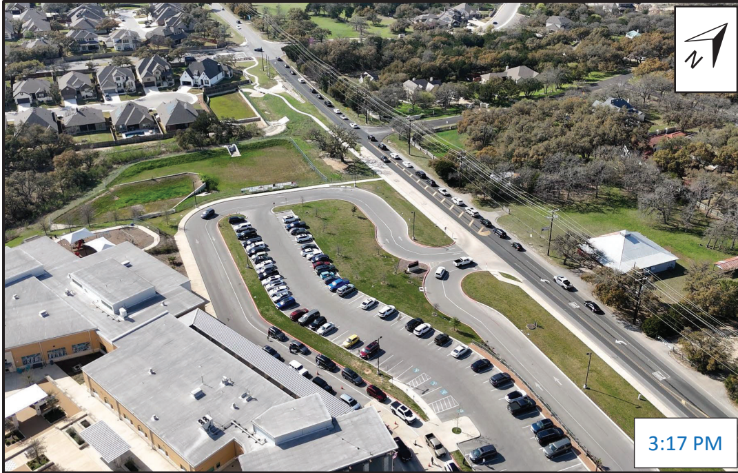
Figure 10 – Approximately 750 LF Queue at Dietz Elkhorn Rd and Square Gate Westbound (PM)
