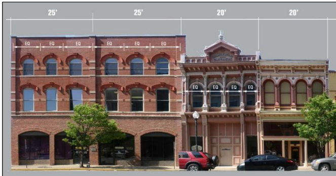
Figure 7-3 Illustration showing building articulation requirement
